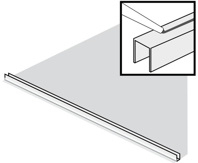
**2** Place the profile on the floor or tray, and mark its position using masking tape.
