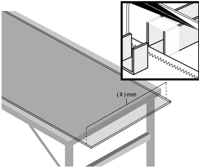
**1** The floor profile is supplied over-length; mark it to the width of the glass with a strip of masking tape. Cut it to length, then file smooth.
