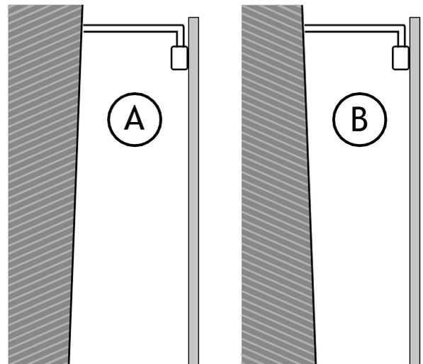
**4** Check that the supporting wall is square; make a note if it is leaning by more than + or - 10mm at the approximate height of the glass. Measure from the inside of the floor profile to the supporting wall (Xmm), and minus 20mm from the figure; then cut the support arm to the calculated length.
